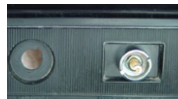
Photo 24. This photo shows the later 1969 -74 Delay Switch and installation hardware. Your switch may look different, depending on the year of your car and type of switch.
