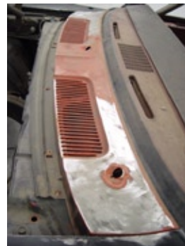
Photo 1. This is the fresh air grille and cowling in front of the windshield opening. Note: in this photo the OEM wiper assembly has already been removed.
