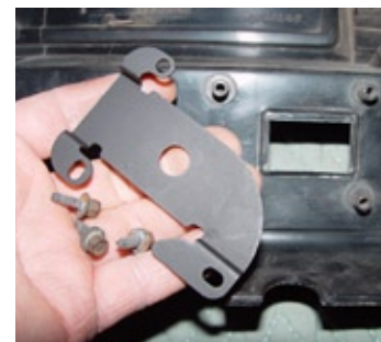
Photo 22. We supply a Rotary Switch Adapter Plate that screws onto the backside of the dash in the same location as the slide switch that came with the car.
