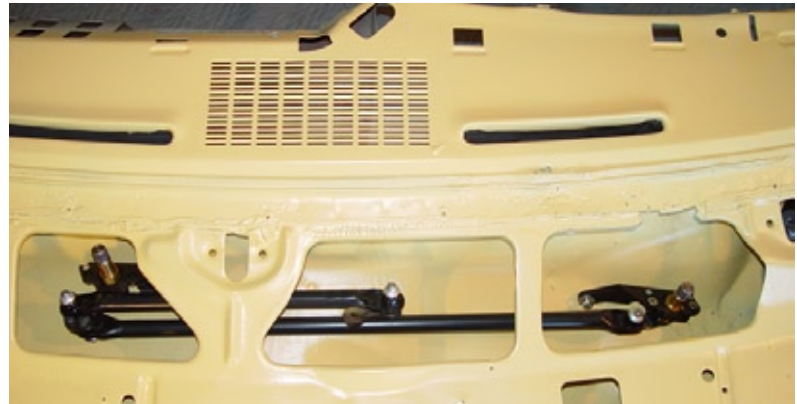
Photo 4. The entire Drive Unit Assembly should end up with the tips of the Pivot Shafts pointing in an upward and aft position. In this photo the Drive Unit Assembly is resting on the bottom of the air box with the Pivot Shafts to the left of their respective pivot shaft openings in the cowl.
