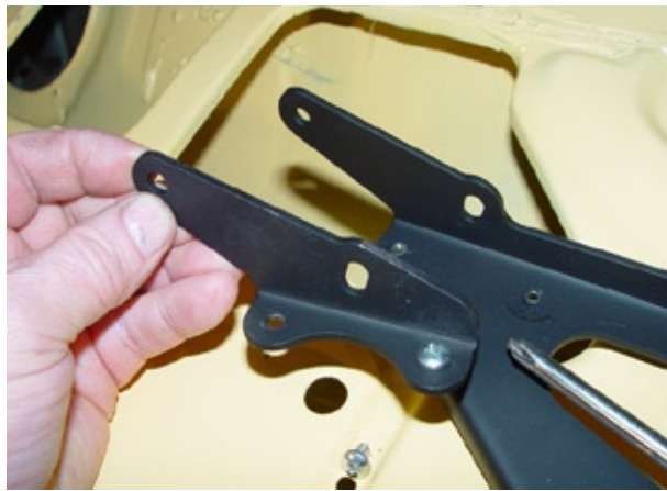
Photo 8. Before putting the Bridge into the air box, attach the Bridge Gusset to the passenger side of the Bridge.
