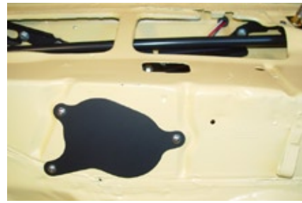
Photo 20. A Cover Plate is provided to plug the motor hole in the firewall if you do not choose to weld it closed.
