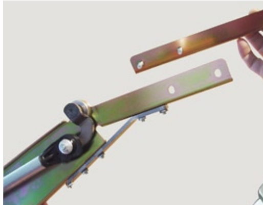
Fig 4: Right - Place the plastic end from the right side cross link onto the top of the first link end on the left side pivot shaft lever. Replace the cup nut on the left side pivot shaft lever.
