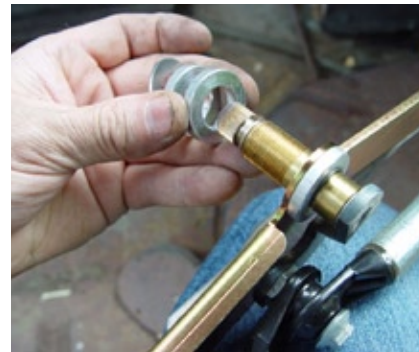
Fig 6: Right- Place 2 of the 4 round spacers then a washer on each pivot shaft before inserting the brass pivot shafts through the stock wiper holes in the cowl.
