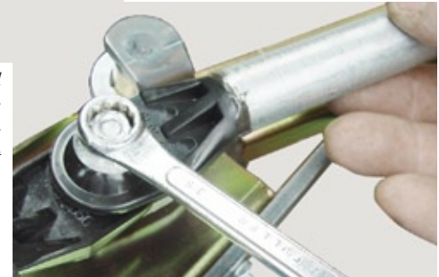
Fig 3: Above - Make sure the right side pivot shaft lever is facing down, similar to the left side pivot shaft lever. The cross link end should be below and slightly to the left of the pivot shaft.
