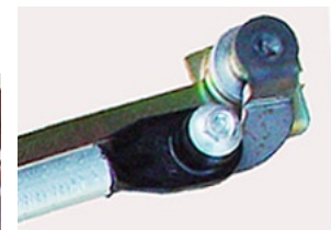
Fig 3: Above - Make sure the right side pivot shaft lever is facing down, similar to the left side pivot shaft lever. The cross link end should be below and slightly to the left of the pivot shaft.
