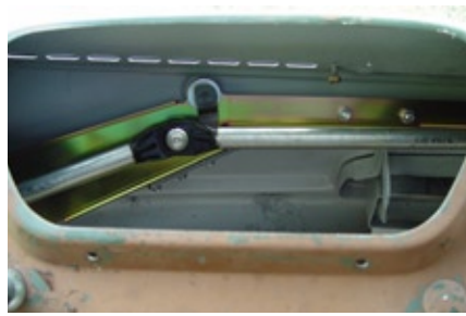
Fig 9: A view of the left pivot shaft, cross link and first link through the gauge cluster opening.
