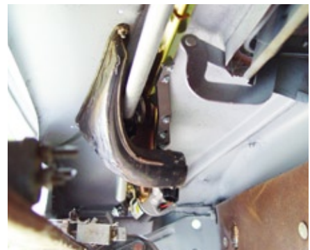
Fig 10: Replace the defroster ducts. The wiper assembly runs between the cowl and the left defroster duct.
