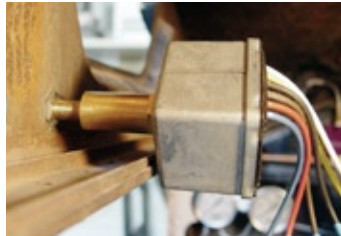
Fig 11: Right- The switches mount in the stock location. Due to the size, the optional variable/intermittant switch is provided with an extension so it will clear the bottom of the dash
