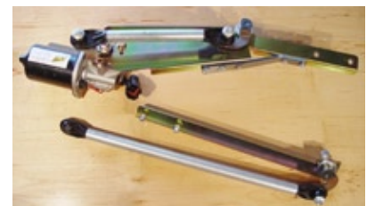
Fig 1: This is the kit as shipped. The one shown is for an F-100 but the F-1 unit is broken down for shipment in the same way.
