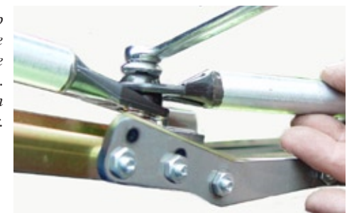
Fig 7: Right - Do not tighten the cup nut too much. Pull up and down on the plastic cup bearing as you tighten the nut. You will feel the play diminish. Remove all play but do NOT tighten the nut any further.
