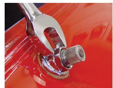
Fig 11: Above- Tighten the chrome nut.
