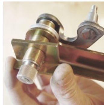
Fig 8: Right- Place the body adapters on both pivot shafts before inserting the brass pivot shafts through the stock wiper holes in the cowl.
