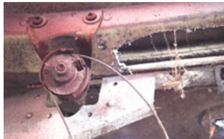
(Fig 03) On 1956-57, remove the spool and cable assembly.
