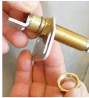
(Fig 21) Add the flat aluminum Pivot Shaft Holding Plate down to the first hex nut and install a second 5/8-24 hex nut.
