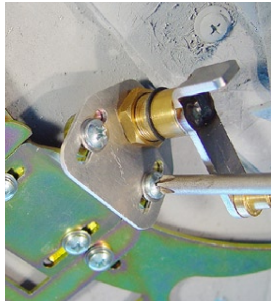
(Fig 81) The other primary, up and down, adjustment is by loosening the two phillips head screws of the aluminum Pivot Shaft Holding Plate so it can be adjusted.
