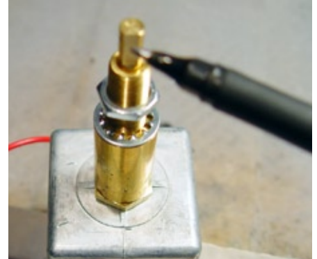
(Fig 111) File enough to allow the set screw to securely clamp the knob to the shaft.
