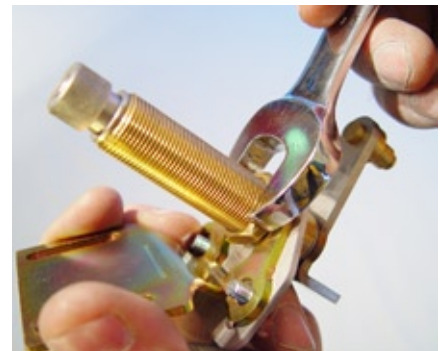
(Fig 33) Run the hex nut down to the Pivot Shaft Orientation Bracket about finger tight.
