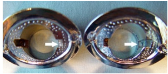
(Fig 11) Each early chrome escutcheon is marked "R" or "L" on the backside down inside the slots.
