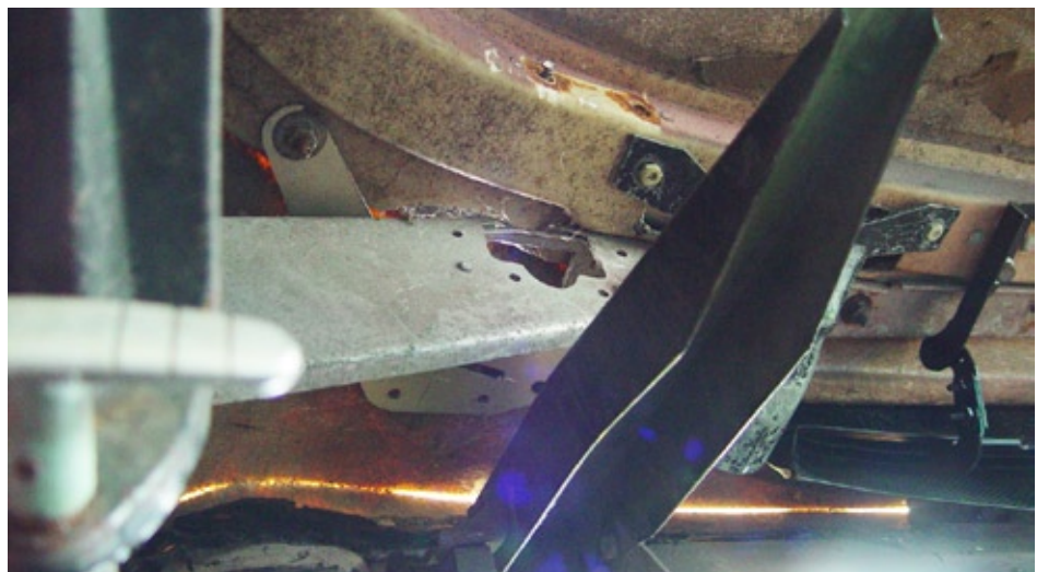
(Fig 72) This shows an early version of the Pivot Shaft Mounting Plate installed above the metal substructure.
