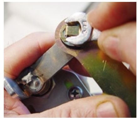
(Fig 93) Using the side of a 1/4 or 5/16 open end wrench or your finger tips, push inward and slide the clip until it snaps in place.
