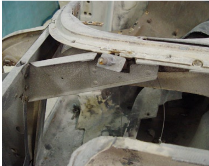
(Fig 70) This is the passenger side looking aft. The fiberglass cowl has been removed. This Corvette has the metal substructure that requires separating the Pivot Shaft Orientation Brackets from the Pivot Shaft Mounting Plates and "U" Guides to install the Pivot Shaft Mounting Plates and "U" Guides between the metal substructure and fiberglass cowl.
