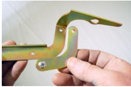
(Fig 50) Attaching the Corner Stiffener to the passenger side Link.
