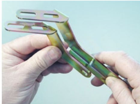
(Fig 55) Match the outer end of the longer Link to the Link End Stiffener.
