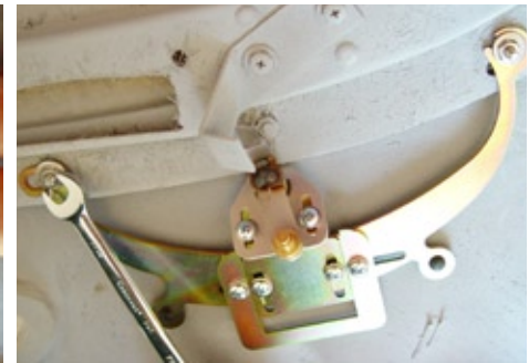
(Fig 76) Place #12-24 hex nuts and 1/4” flat washers on the windshield retaining studs and tighten them.
