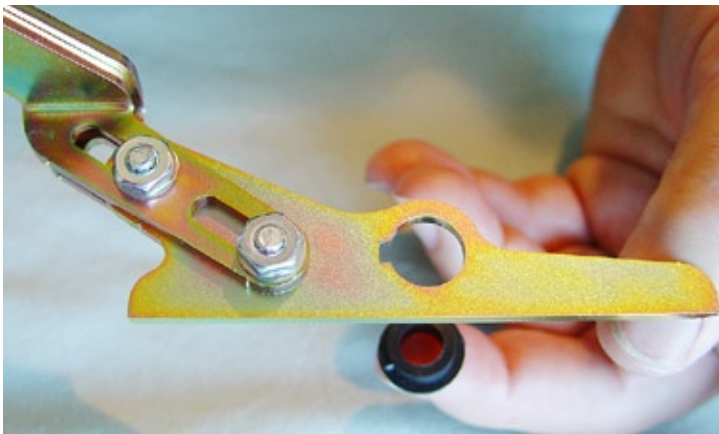
(Fig 63) Push the Plastic Bushing into the keyed hole as far as it will go.
