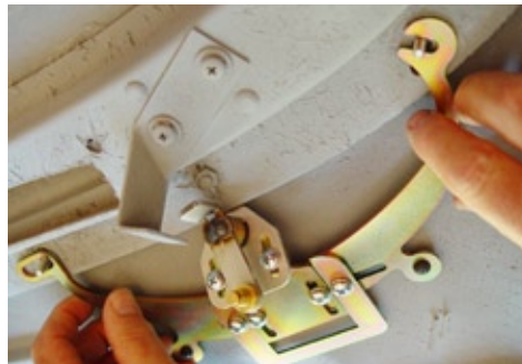
(Fig 75) You can install the pivot shaft mounting assembly as a single unit on cars without the metal sub structure. This photo shows the passenger’s side.
