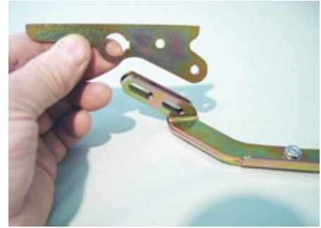
(Fig 56) Sandwich the Link Tip between the Link and the Link End Stiffener.
