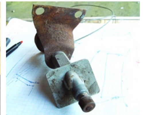
(Fig 06) The pivot shaft after being removed.
