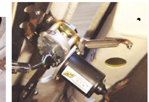
(Fig 45) The opposite end of the Motor Brace goes up against the underside of the firewall where the left side of the old (OEM) wiper motor was attached. Attach the Brace using a 10-32x3/4" phillips, washer, and nut. This same fastener holds one side of the new Cover Plate.
