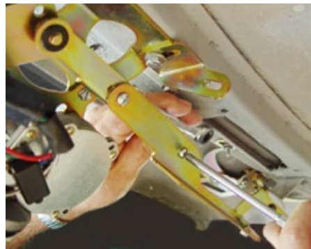
(Fig 90) Passenger side Link length adjustment. Loosen the two phillips head screws that attach the long and short Link halves. Slide them apart or together to adjust the length.
