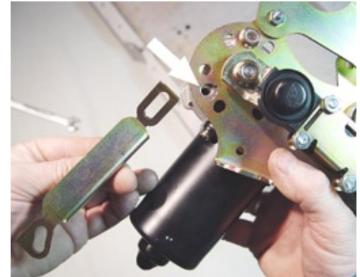
(Fig 41) Use a 10mm wrench to remove the motor mounting screw as shown
