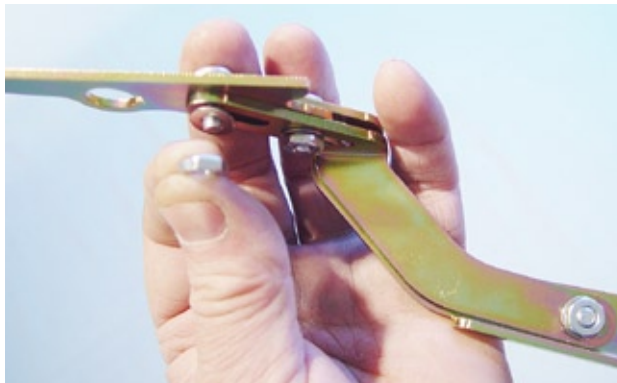
(Fig 55) Match the outer end of the longer Link to the Link End Stiffener.
