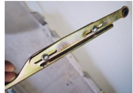
(Fig 58) Attach the short Link to the other end of the longer Link assembly.
