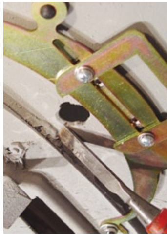
(Fig 73) Some Corvettes need the excess glue, aft of the pivot shaft, removed so the new pivot shaft will fit properly.
