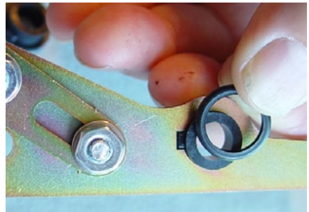
(Fig 64) The Plastic Bushings that fit into the keyed holes in the Link Tips have a plastic ring that fits on the side that extends through the keyed hole.
