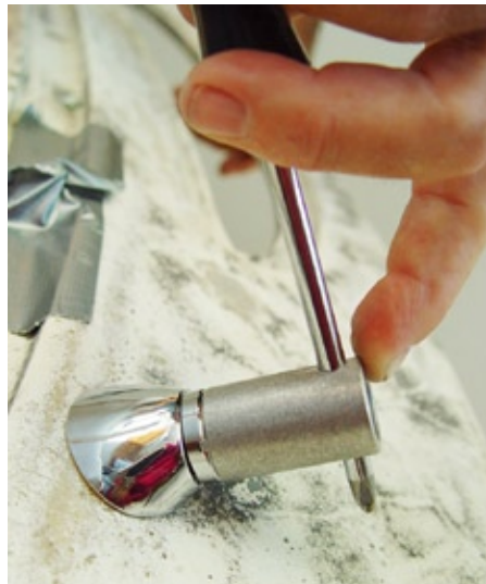
(Fig 84 & 85) When you are satisfied with the fit of the Pivot Shaft and chrome escutcheon fit on the outside of the car, tighten all interior screws before installing the chrome escutcheon nut with the aluminum Escutcheon Wrench supplied in the kit. Overtightening can damage the fiberglass.
