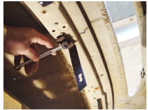
(Fig 02) Remove the radio support.
