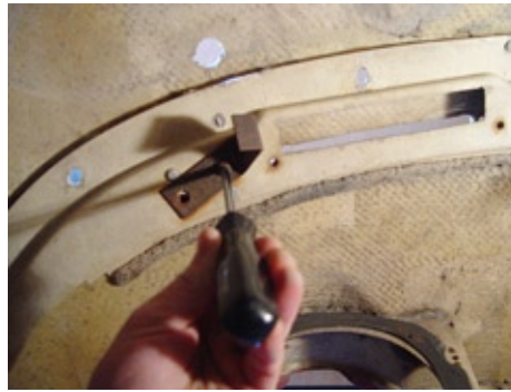
(Fig 01) On 53-55 Corvettes you do not need to remove the stock pivot shaft brackets. On 1956-62 Corvettes you do.
