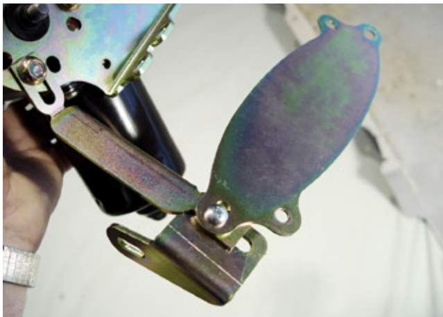
(Fig 103) This photo illustrates how the Motor Brace, Windshield Brace Mounting Bracket and Cover Plate share the same mounting point.
