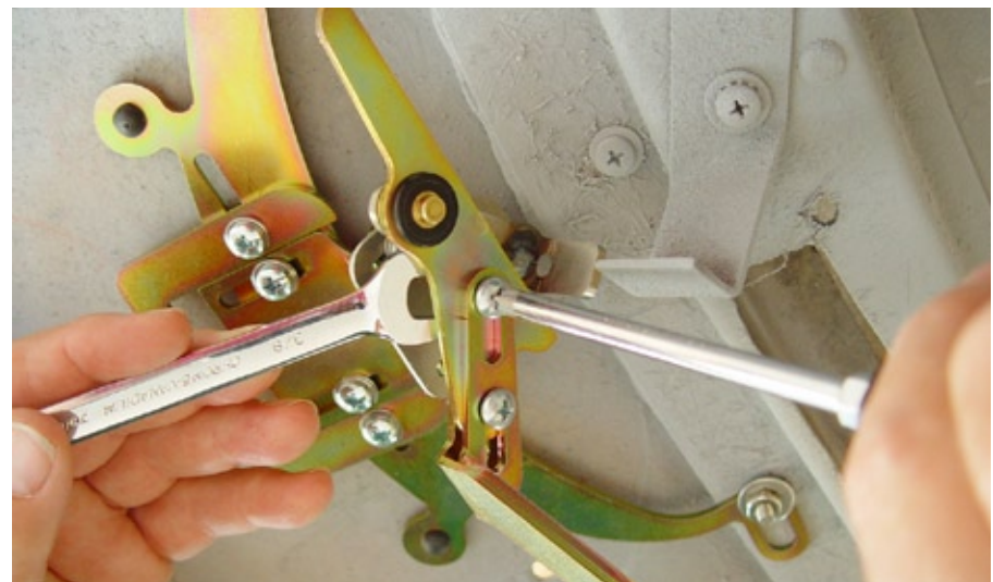
(Fig 95) On the driver side loosen the two phillips head screws, extend or retract the Link Tip as needed clear both the defroster duct and the brake pedal/clutch pedal bracket. Retighten the screws.
