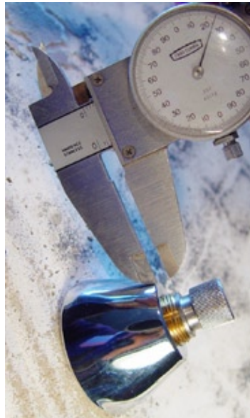
(Fig 79) With the chrome escutcheon placed onto the Pivot Shaft and resting on the body, 1/8" to 3/16" of the brass threads of the Pivot Shaft should be showing.
