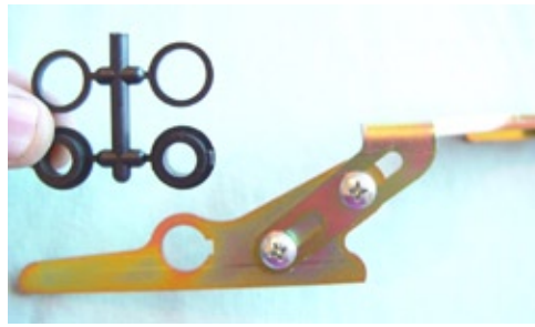
(Fig 60) The Plastic Bushings that fit into the keyed holes in the Link Tips & opposite Link ends.
