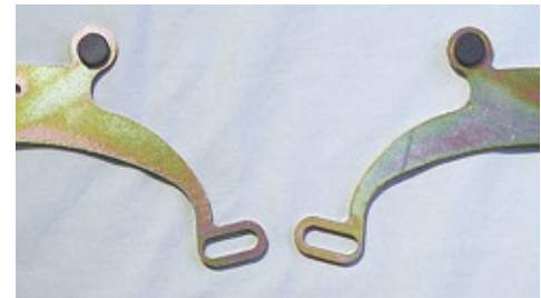
(Fig 15) The bumpers have been installed on the top of both brackets.
