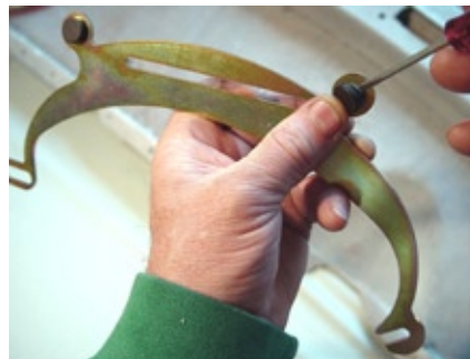
(Fig 14) Using a small tip screwdriver, install 2 rubber bumpers in each part so that the bumpers for each part is on the top side.
