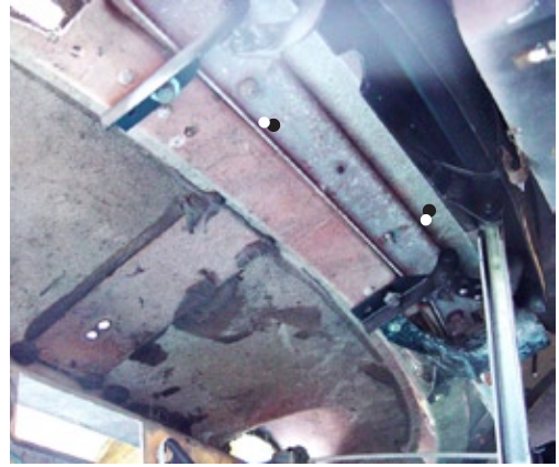
(Fig 43) Remove 4 1/4-20 hex bolts holding the cowl vent hinge brackets to the under side of the cowl.
