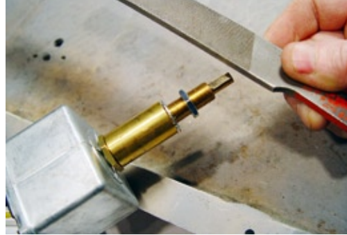
(fig 110) File a flat spot in the shaft at the 6 o'clock position for the switch knob's set screw.
