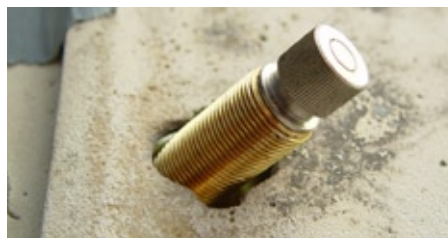
(Fig 77) The Pivot Shaft should be centered within the hole in the cowl.
