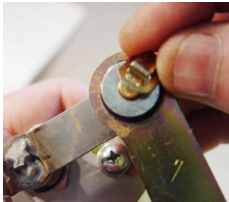
(Fig 92) Place a thin washer and spring clip onto the exposed end of the upper brass pivot pin on the Drive Unit.
