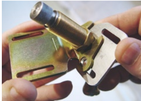
(Fig 30) Slip the tips of the open end of the Pivot Shaft Orientation Bracket onto the brass Pivot Shaft.
