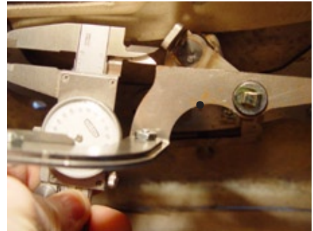
(Fig 91) When the Pivot Shaft is in the parked position, there should be between a 1/4" to 3/16" gap between the flat in the Cross Link end and the stop tab on the Pivot Shaft.
