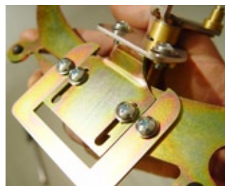
(Fig 32) Using two 10-32x3/8" phillips head screws and flat washers, attach the aluminum Pivot Shaft Holding Plate to the Pivot Shaft Orientation Bracket.
