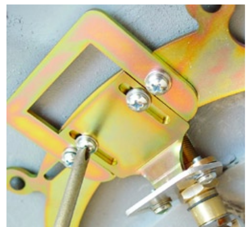
(Fig 78) A primary adjustment is by loosening the four phillips head screws in the Pivot Shaft Orientation Bracket. The inside two give front to back (in and out) adjustment. The outside two give side to side adjustment.
