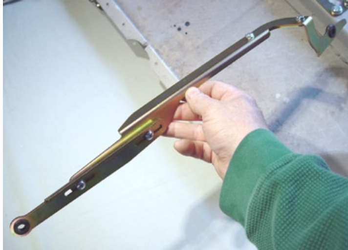
(Fig 50) Attaching the Corner Stiffener to the passenger side Link.
